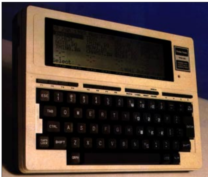
Looking back at the future: Tough and eminently usable, the M100's four AA batteries gave a whole week of service, unlike today's notebooks where a measly three hours is the norm
